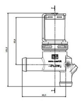
Suitable for applications using water at temperatures up to 90°C (194°F)
