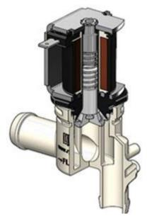
The Pilot-operated diaphragm provides high flow capacity with minimum power requirements and its unique diaphragm design reduces unwanted particles from entering the armature area, minimize the possibility of jamming due to foreign materials.
